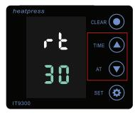
Press ↑ & ↓ button to determine the Temp. will be modified, Say. 30F (i.e. heating platen 30F hotter than the gauge read-out)
