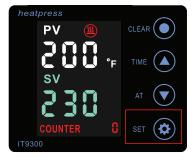
Press SET key to back to window and read-out 200F, and heat press will continue to heat up to 230F
