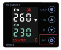
Press SET key to go back to window and read-out 260F, and heat press will cool down to 230F
