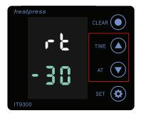
Press↑ & ↓ button to determine the Temp. will be modified, Say -30F (i.e. heating platen 30F cooler than the gauge read-out)
